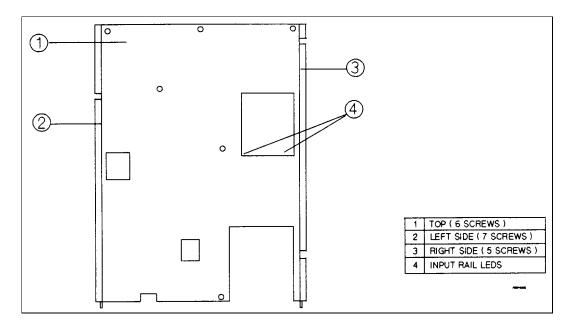
Figure C-4. Removing the Series 668xA Inner Cover
